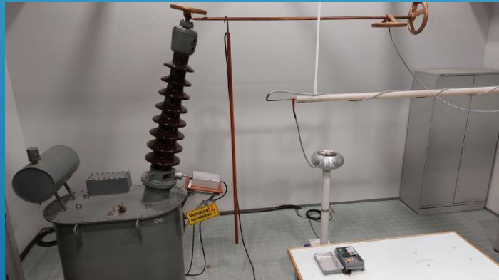
Fig. 6. Capacitive energy harvesting from high voltage power lines.
