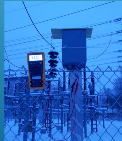
Fig. 6. Capacitive energy harvesting from high voltage power lines.
