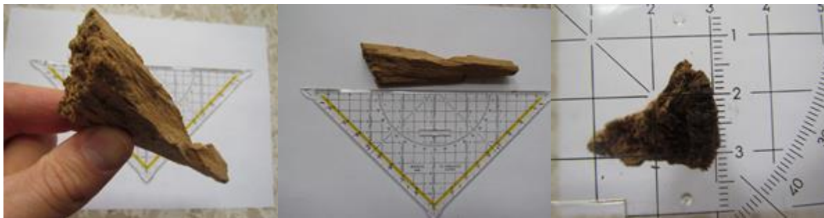
Figure 3. Measuring the cross section area of the largest particle using a set square. The measurement result is around 2.25 \text{ cm}^2 . Photos: Holzforschung Austria.
