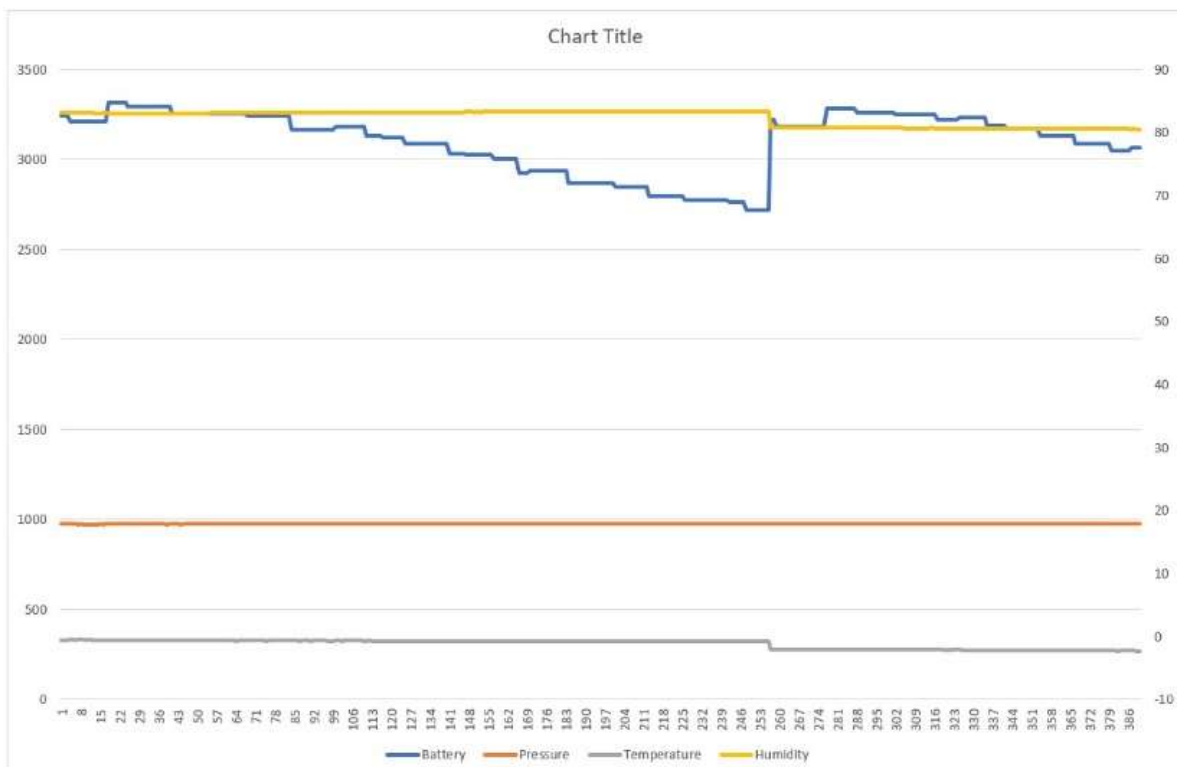
Figure 2.2.4.3 Battery voltage (blue), air pressure (orange), air temperature (gray) and humidity (yellow) at the different data points during the test period. The x-line is the sequence of data points.
