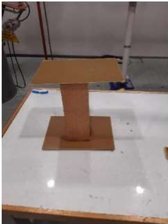
Figure 2.2.2.2 Test arrangement for harvester plates. The distance between the copper plates is 30 cm. The size of the copper plate is 30 cm x 21 cm. The overhead power line is cut out of the figure. The power line is about 1.2 m above the upper copper plate.
