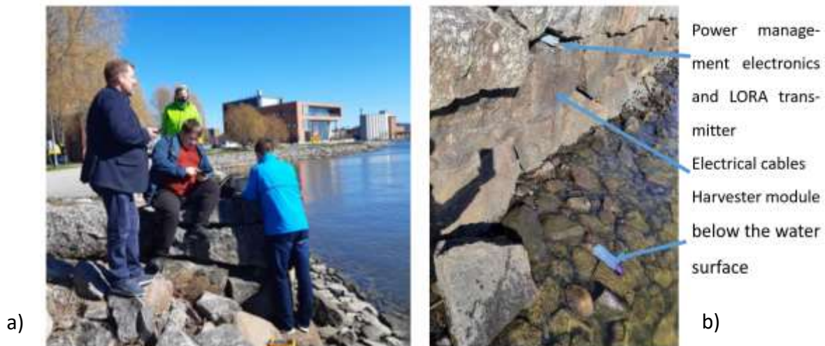
Figure 6.8.1 Measurement of the efficiency of the harvesters in seawater. a) Preparation of the field measurements of the electrochemical harvesters in seawater. b) Position of the harvester module and the power management electronics in the test area.
