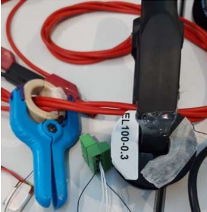
Figure 3.1.3 The tested inductive harvesting coil structures. First, the right with full winding wire rolls and round split ferrite from the EMC laboratory glued to a plastic grip, then the left later used ferrite cut in two halves with wire wound around one of the halves.
