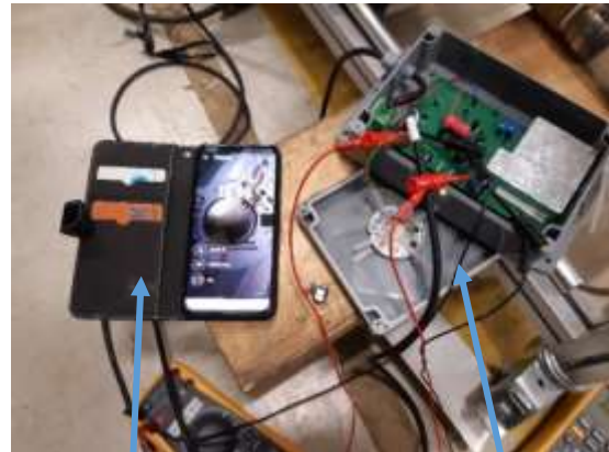
b) Phone as the data receiver and energy harvesting electronics
