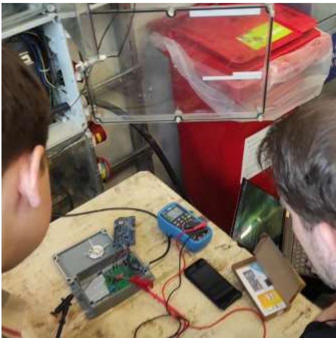
Figure 3.3.8 Measurement at Viimatech Digital Oy powering the nrf9160 development kit
