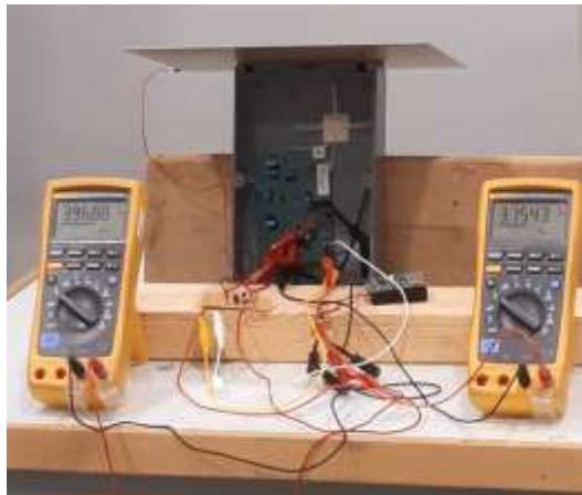
Figure 2.2.3.1 Test arrangement for Version three of the energy harvester circuit and energy management. The top of the electronic box is a 21 cm x 30 cm Cu plate that is the harvesting module. The voltage meters are measuring the input voltage and battery voltage. The left circuit on a wood block is the voltage regulator, and the right circuit is an IoT device.
