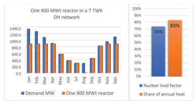
As we can see, the single 900 MWt reactor would run at a suboptimal 74 % load factor, but it would supply 83 % of the total heat demand. The BWRX-300, the only reactor of this size presented in this study, is suitable for electricity production as well (at 300 MWe), so it would make more sense to run it at combined heat and power. With CHP, there might be room for a second unit as well.
