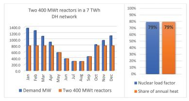
Two 400 MWt DH reactors, like the DHR400 from China, manage to run at almost 80 % capacity factor and produce almost 80 % of the energy demand, while adding redundancy compared to the case with a single larger reactor. A similar, even more flexible setup could be achieved with four 200 MWt reactors.
