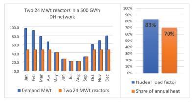
The two 24 MWt reactors would run at reasonable 83 % load factor, as their annual maintenance periods can be timed optimally for July and August, the months with the lowest demand. The reactors would produce around 70 percent of the total annual heat demand. Two reactors would also improve redundancy, as if one would shut down for some reason, the other could go on producing heat.
