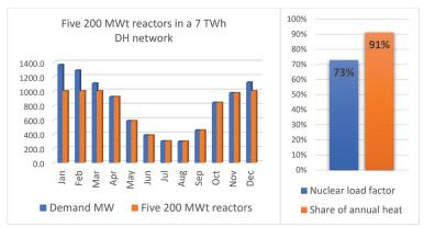
As an extreme case, five 200 MWt heating reactors running in 7 TWh network manage to produce over 90 % of the required heat, while running at 73 % load factor. This configuration would al-
