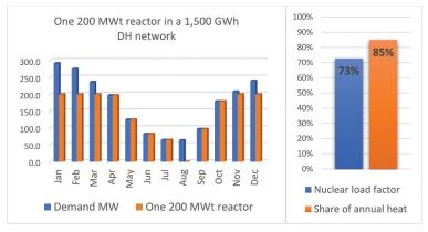
A single 200 MWt reactor would provide 85 % of the annual heat demand but would work at a somewhat low 73 % load factor, with scheduled maintenance in July or August. It would also be a rather big single source of energy, when considering security of supply. A single heat-only reactor would likely have lower O&M costs so that could mitigate the low load factor.
