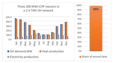
To produce all of the heat demand of a 2.4 TWh annual demand city such as Turku, Tampere or Espoo, three 200MWt CHP reactors could be used. In addition to the heat, they would produce 0.7 TWh of electricity as well.
