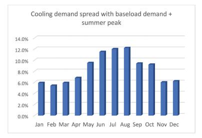
District cooling is sold around the year, and is used at sites like data-centres, while summer-time (May to October) has a peak in demand as residential buildings are also cooled. This peak can be handled by the otherwise un-used nuclear heat capacity, which will increase the load factor of the reactor by a couple percentage points, depending on the situation. The above graph of the monthly demand variation of cooling is for illustrative purposes (not exact data).
