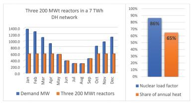
Three 200 MWt district heating reactors, such as SECURE, HAPPY or NHR200-II, would be able to operate at a rather optimal load factor of 86 % and produce two thirds of the annual heat demand.
