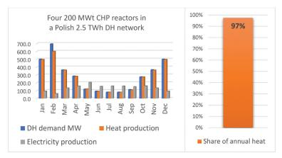
With CHP enabled (using the same parameters as we did previously), a set of four 200 MWt reactors (such as the NuScale) would produce practically all the heating demand, and 1.2 TWh of electricity.
