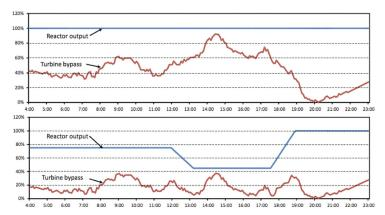
Figure 6 Two load following options for NuScale. Above is turbine bypass only. Below is turbine bypass and reactor power manoeuvring in combination.
