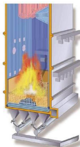
Picture 3.2. BFB boiler furnace (Valmet Ltd)
